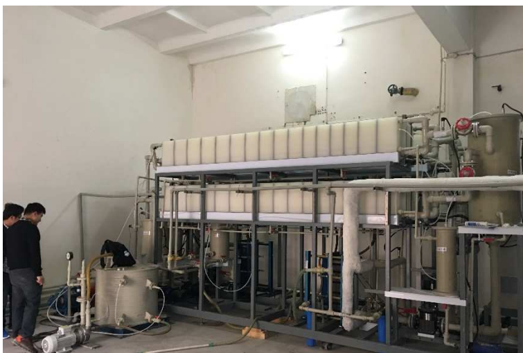
Actual MDS 2000 system for NH 4 Cl concentration in food industry
